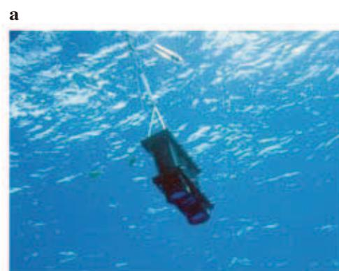
**Fig. 18.** A compact underwater digital movie camera system developed in 2003, a: a view from below, (Photo by K. Mori)
