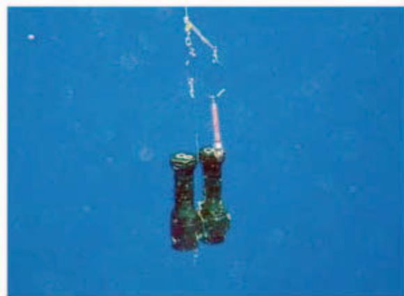
**Fig. 3.** Remote camera system with under-water pencil light. (Photo by K.Mori)
