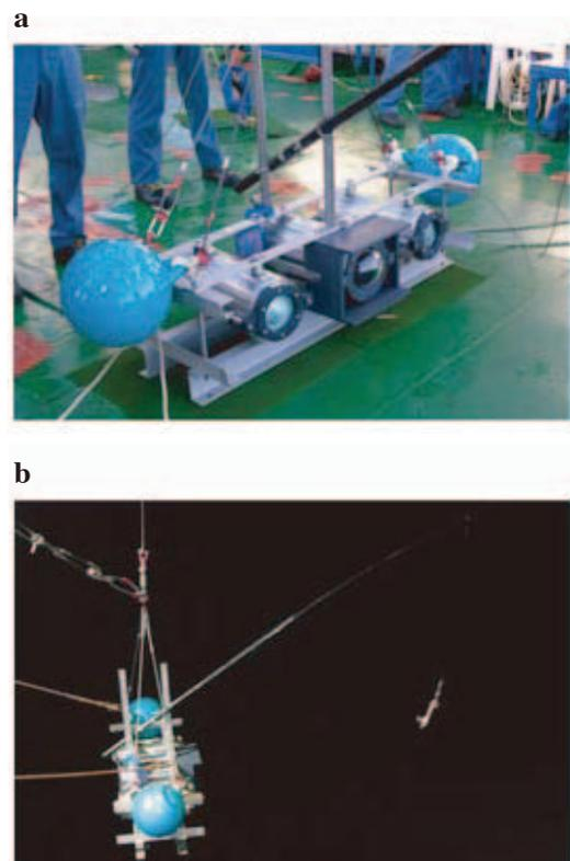
**Fig.19.** A new underwater high definition video camera system developed in 2005, a: camera system on deck, b: system with pole and bait rig.
