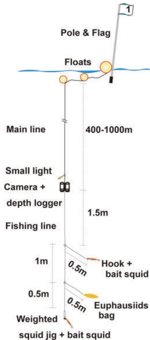
Fig. 4. Diagram of vertical long-line system used for survey.
